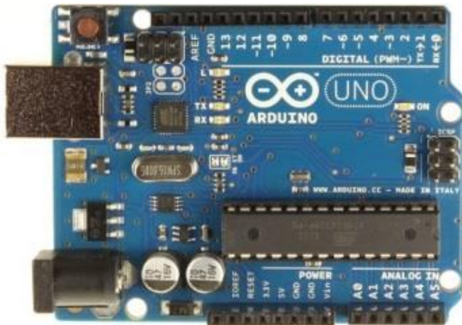
Arduino UNO R3 board with ATmega328P – ( Click to see on Amazon http://amzn.to/YMjZq )
